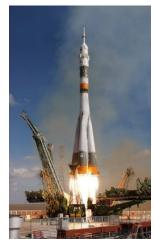
**Answer:** Most of the rockets that are used to launch satellites into orbit have two stages. The first stage must be powerful enough to carry the rocket and its payload through the thickest part of the Earth's atmosphere.
