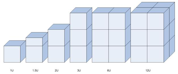
The use of standard sizes and shapes makes it relatively easy to adapt launch vehicles and their deployment mechanisms to carry a payload of CubeSats. Most CubeSats are 3U, 6U or 12U.
