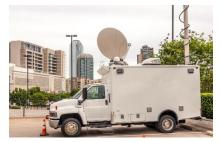
Ground stations can be built into vehicles and used to provide mobile satellite communications. For example, a television broadcaster might use a truck equipped with a dish and communications equipment to transmit live video via satellite from a sports event back to the studio from which it will be retransmitted to viewers.
