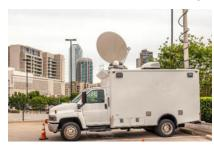
Ground stations can be built into vehicles and used to provide mobile satellite communications. For example, a television broadcaster might use a truck equipped with a dish and communications equipment to transmit live video via satellite from a sports event back to the studio from which it will be retransmitted to viewers.
