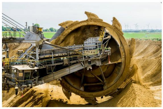
Hard rock deposits of lithium are mined mainly by the open pit method. Blocks of rock containing lithium are dug out of the earth. They are then crushed and milled to create a fine powder. The powdered rock is mixed with water. Bubbles of air are injected into the mixture. The bubbles attract lithium while they rise to the water's surface. The resulting foam is skimmed off and sent to a plant where it is processed to produce lithium carbonate.
