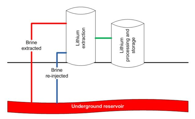
This process is essentially an alternative to traditional brine mines. It is more expensive, but it avoids the environmental damage associated with storing brine in evaporation ponds. It also uses solvents to extract the lithium from the brine, so the extraction plants use much less fresh water.
