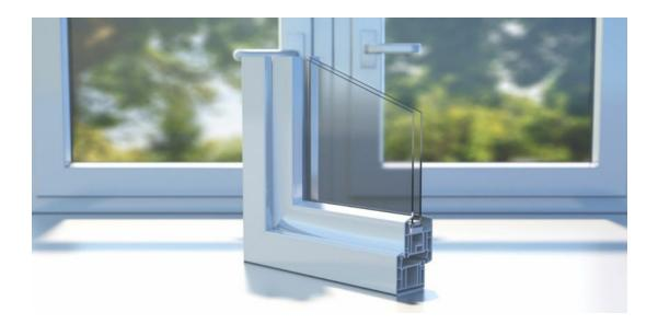
The glass used in double glazing is supplied in the form of sealed units. A sealed unit consists of two panes of glass that are joined around their edges by a spacer bar. The glass and spacer bar are held together using adhesive that creates a solid seal.
