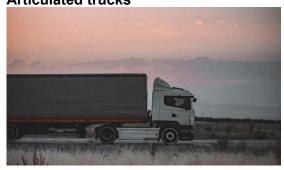
Articulated trucks consist of a tractor unit and a trailer. The tractor unit has the driver's cab, the engine and the fuel tanks. The trailer carries the load.
