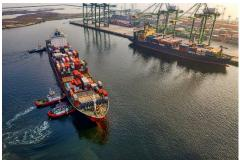
Container ships carry goods in shipping containers, which allow for rapid loading and unloading. Many ports have container terminals that are equipped with cranes designed to lift containers. Once unloaded, containers can be stacked ready to reload onto another ship. Containers can also be loaded onto trucks or trains. Containers are standard sizes, which makes them easy to manage.
