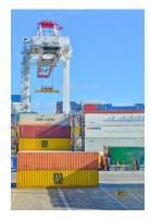
Intermodal transport frequently involves freight that is being carried in shipping containers. These can be stacked on the decks of container ships or loaded onto wagons on freight trains or trailers on articulated trucks. The containers can also be stacked on land for storage purposes, enabling goods to be stored without the need for warehouse space to protect them.
