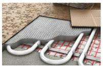
Underfloor heating is an alternative to radiators. Hot water from the boiler is piped from room to room. Plastic pipes are set into the concrete floor in a zigzag design that enables heat to be released, creating an even heat across the whole room and avoiding the need to install radiators on the walls of the room.
