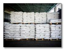
When they are required for production, the paper sacks are transported mechanically and emptied into massive metal drums, with the number of sacks from each batch of black tea specified by the tea blenders. The drums rotate slowly until the leaves from each batch have been mixed evenly. A sample is tasted by the factory's quality control technicians to confirm that the mixture of leaves in the drum is satisfactory before any further processing.
