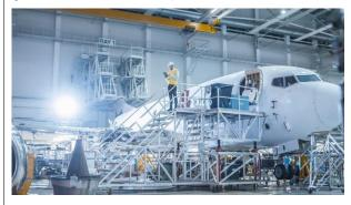
Major repairs are carried out in a hangar. Hangars are huge buildings that can accommodate a whole aircraft and still leave sufficient space to build work platforms and allow major parts such as replacement engines to be brought in.
