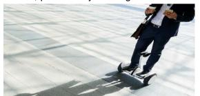
the two wheels. The hoverboard is controlled by the operator leaning in the desired direction of travel. A slight lean forward makes the machine roll ahead and leaning to the left or right makes the machine turn in that direction. Leaning backward will make the hoverboard slow down and reverse if the operator continues to lean in that direction after stopping.
