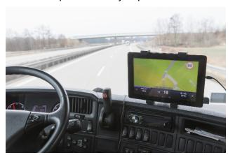
Runn's vans are fitted with electronic systems that are integrated and fulfil a number of functions automatically, without the driver being distracted while driving. A computer is built into the dashboard of each van. The computer uses mobile phone technology to exchange data with the depot and Bluetooth to exchange data with the driver's handheld scanner. The computer also has an integrated satellite navigation system.
