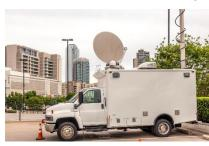
Ground stations can be built into vehicles and used to provide mobile satellite communications. For example, a television broadcaster might use a truck equipped with a dish and communications equipment to transmit live video via satellite from a sports event back to the studio from which it will be retransmitted to viewers.
